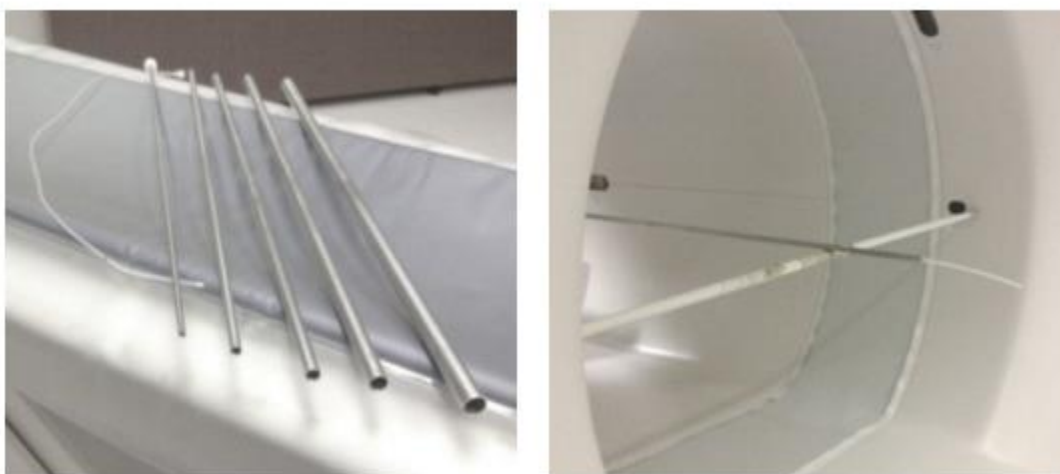
Figure 2. Example of a fantoma sensitivity for PET with various sizes of tubes with different activities.
