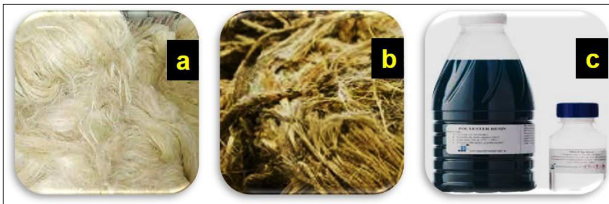
Fig.1. Photographic Images of (a) Sisal; (b) Kenaf and (c) Polyester Matrix
