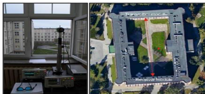
Figure 11. Outside the Military University of Technology building, the laboratory is used to test the electromagnetic link.
