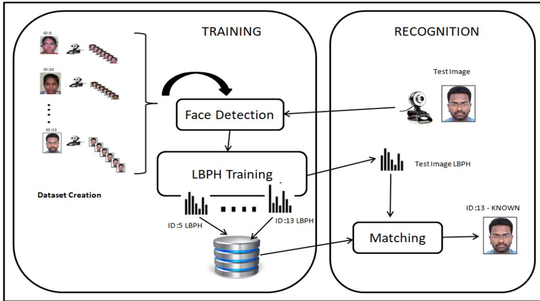
Figure 2 The Block diagram of the Recognition Module
