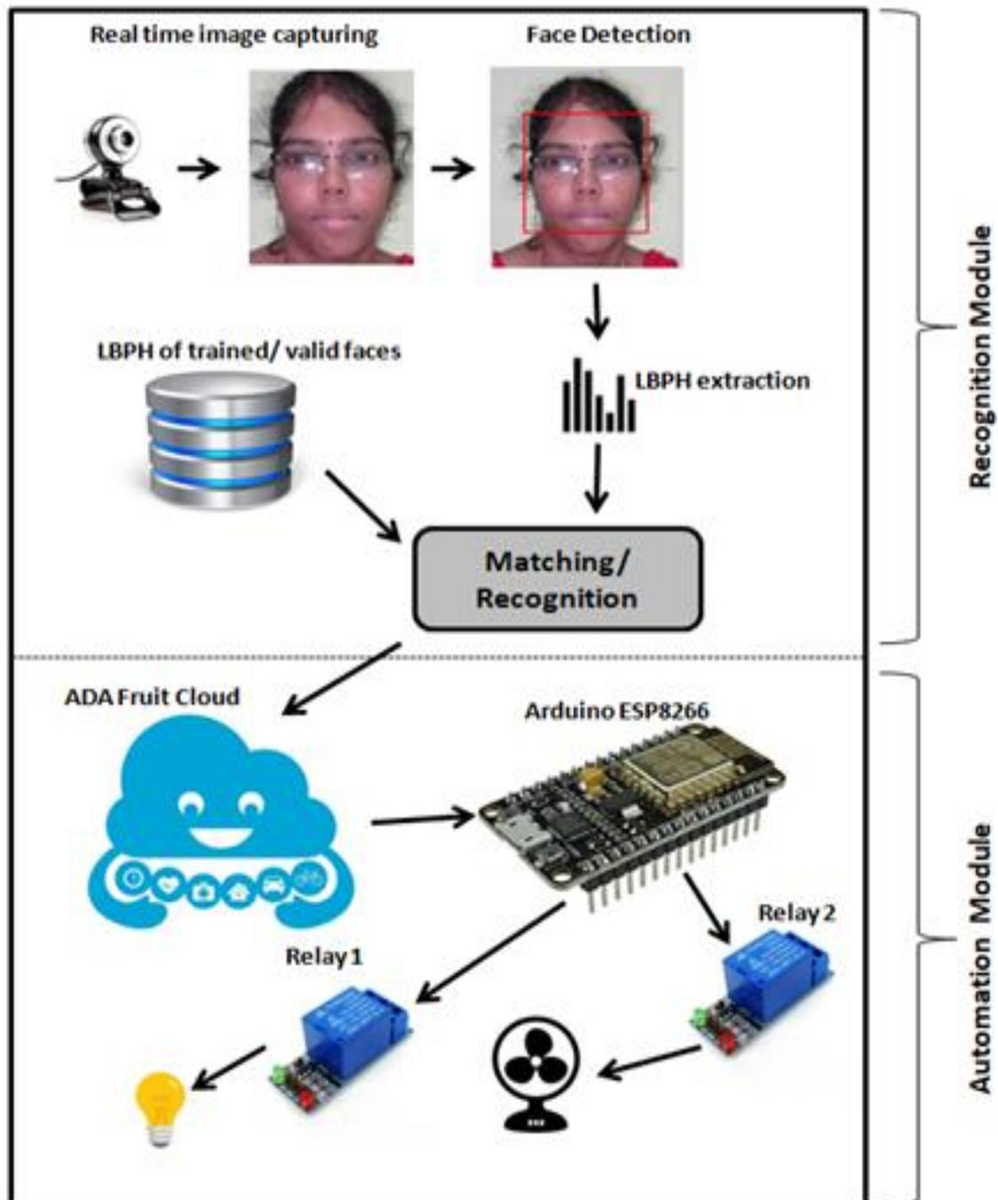
Figure 1 The proposed real-time office automation system
