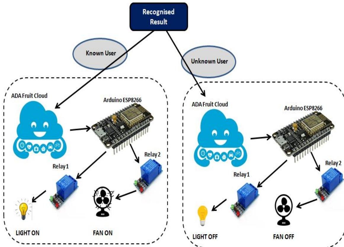
Figure 6 The Block diagram of the Automation Module
