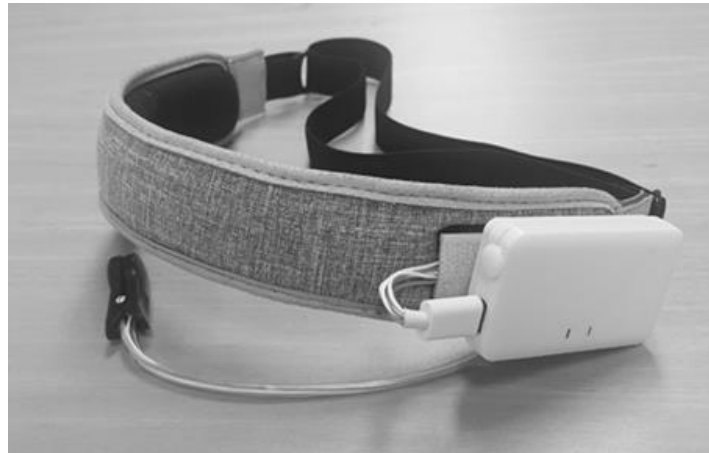
Figure 2. Measuring Equipment for Detecting the Biosignals of the Subjects
