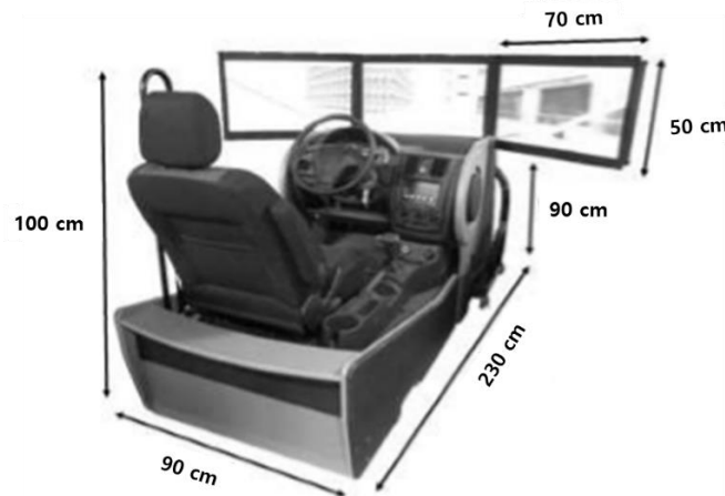
Figure 1. Graphic Driving Simulator Used in this Study
