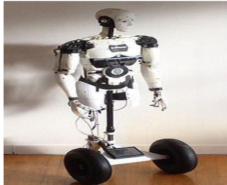
Fig.1: UV-C based humanoid robot with automatic spraying mechanism [1]
