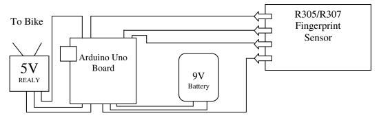
FIGURE 1 From left to right in this diagram there are 4 components first one is Arduini UNO board, Finger Print, One Channel Relay (v battery AS shown in figure
