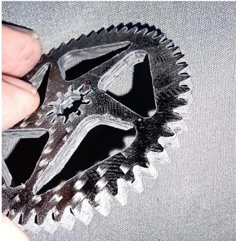
Figure 10. Gear profile cut out from carbon fiber sheets
